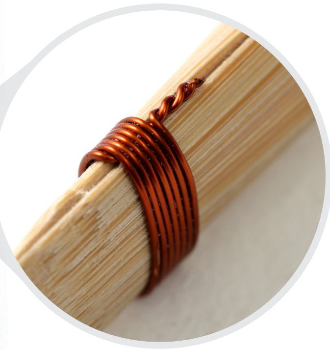
The top of the 'Seo' is coiled with a thin copper wire.
